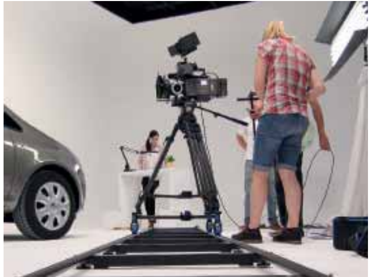
Above: Kombidolly with tripod on the Kliktrak rails Below: Kombidolly using studio wheels with camera head mounted on lo-bowl adapter
